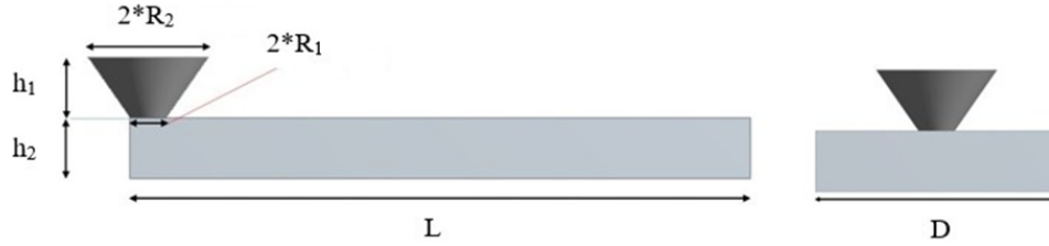
Figure 2. Model abrasive particles and workpiece
